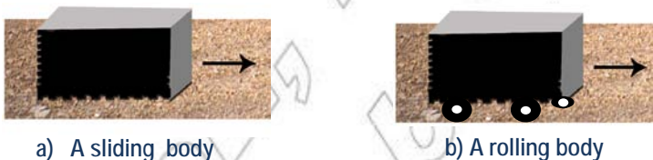
Fig 3.18 Rolling reduces friction
